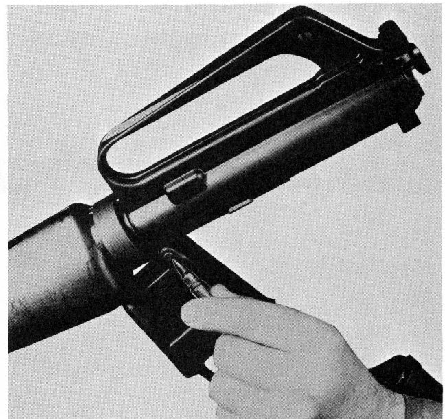
29,352 Figure 11-27. — Pressing out receiver pivot pin.
